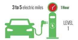
**Level 1 charging:** Provides the slowest charge, around 3 to 5 electric miles per hour. Even at this slow speed, however, the majority of electric vehicle owners plug in at home to refuel.
